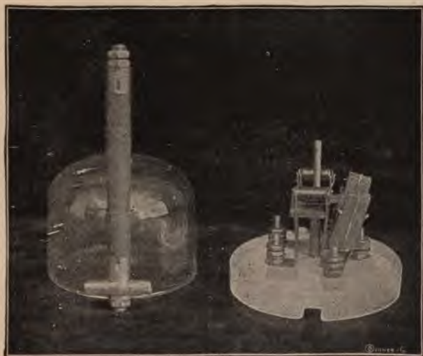
FIG. 221.—Sterling combined heat coils and carbon arresters for protecting a subscriber's station apparatus; also long tubular fuse for protection on the line outside the subscriber's station.
